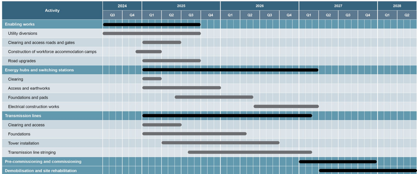
Figure A-13 Indicative construction program
