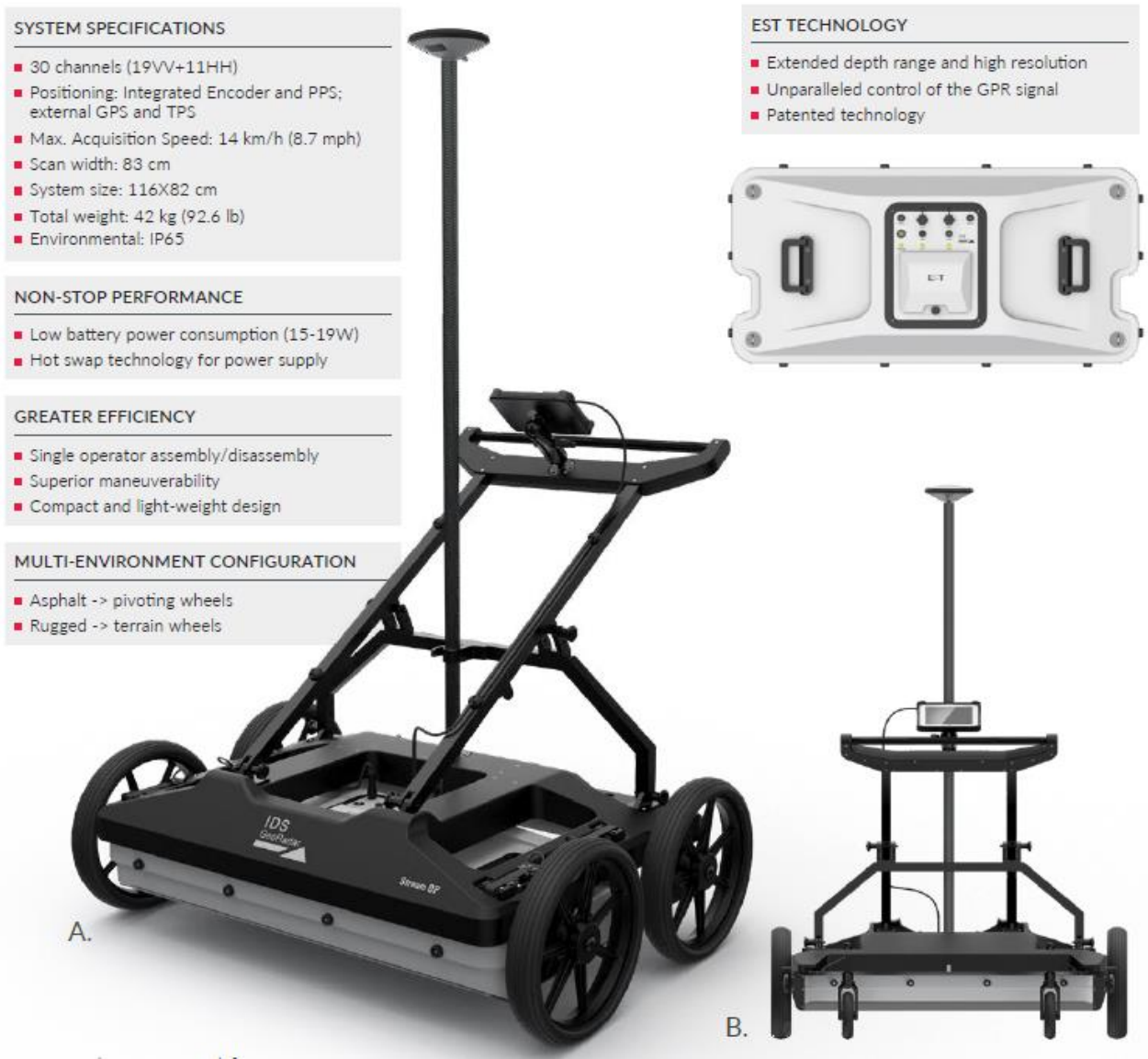
Figure 2: Ground Penetrating Radar used onsite.
