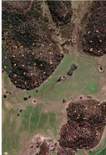
Photo 5-1 Example of two-phase grid-based systematic survey methods using a pre-loaded handheld GPS (orange dots = 40 metre diameter search, white dots = preloaded 100 metre grid points)
